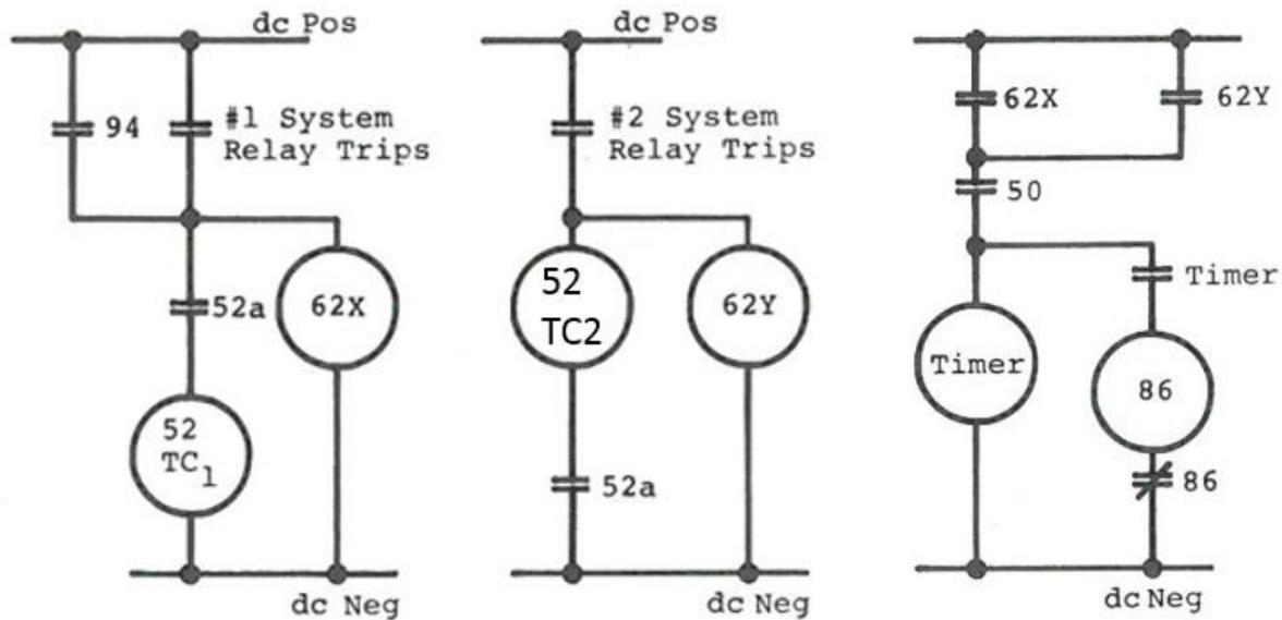
*Scheme 2: Breaker Failure Protection Scheme in Electromechanical Based Relays*
