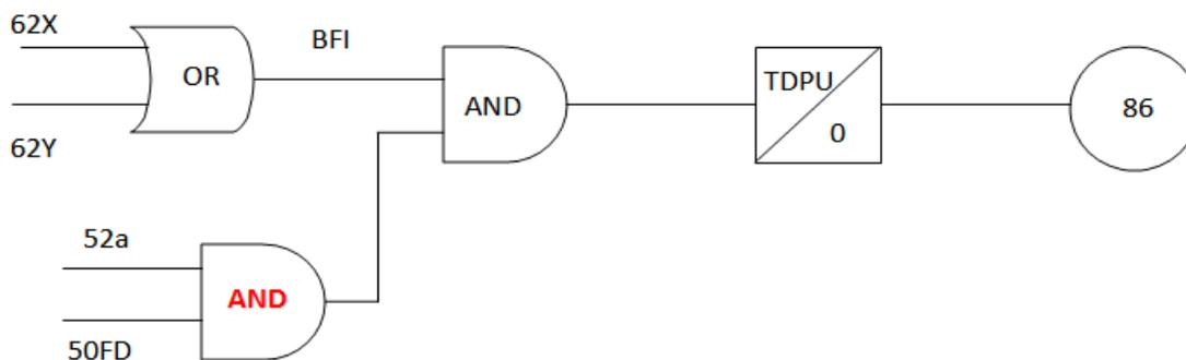
*Figure 2: Breaker failure Logic Using 52a Contact AND with Current Detector*
