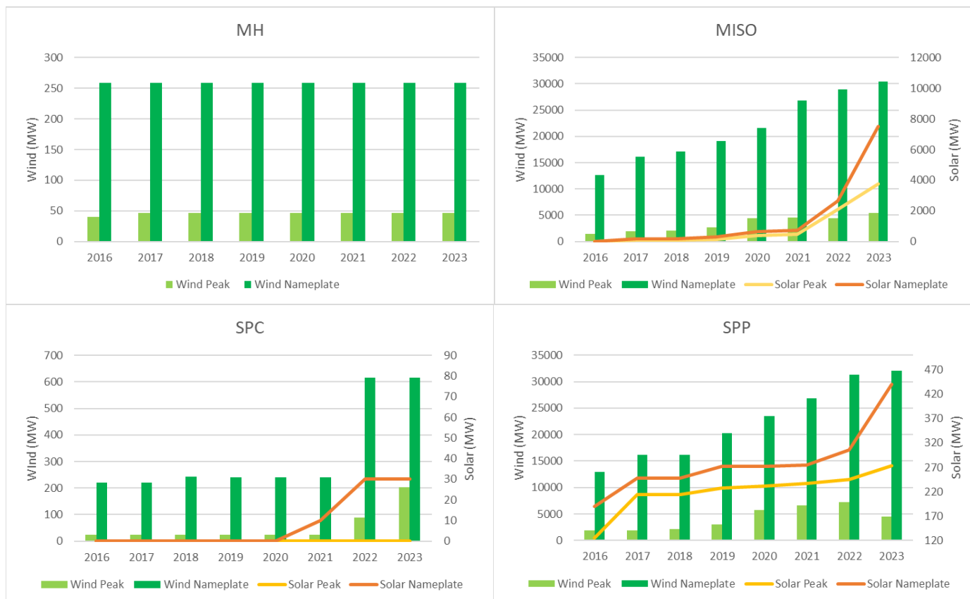
Figure F2: Wind and Solar Photovoltaic Nameplate and Peak Capacity
