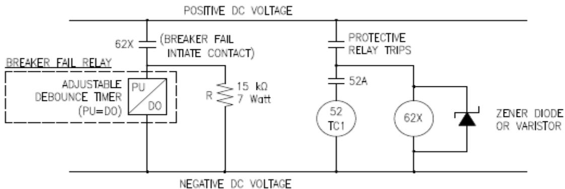
*Figure 3: Breaker Failure Scheme with Adjustable Timer*
