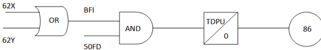
***Scheme 1: Breaker Failure Protection Logics in Microprocessor Based Relays***
