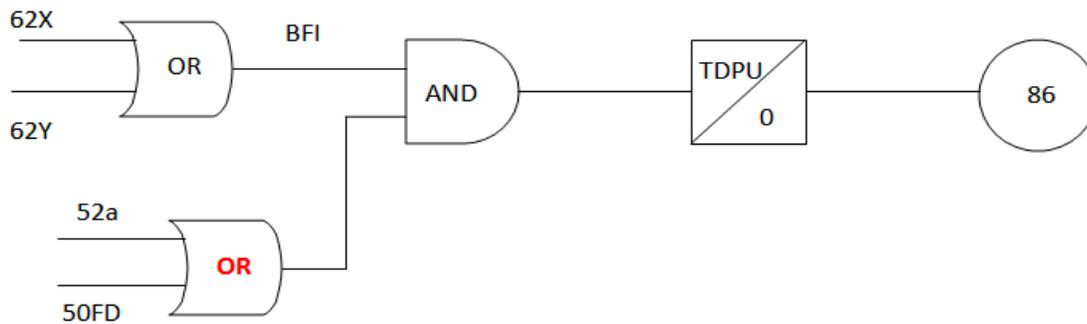
*Figure 1: Breaker failure Logic Using 52a Contact OR with Current Detector*
