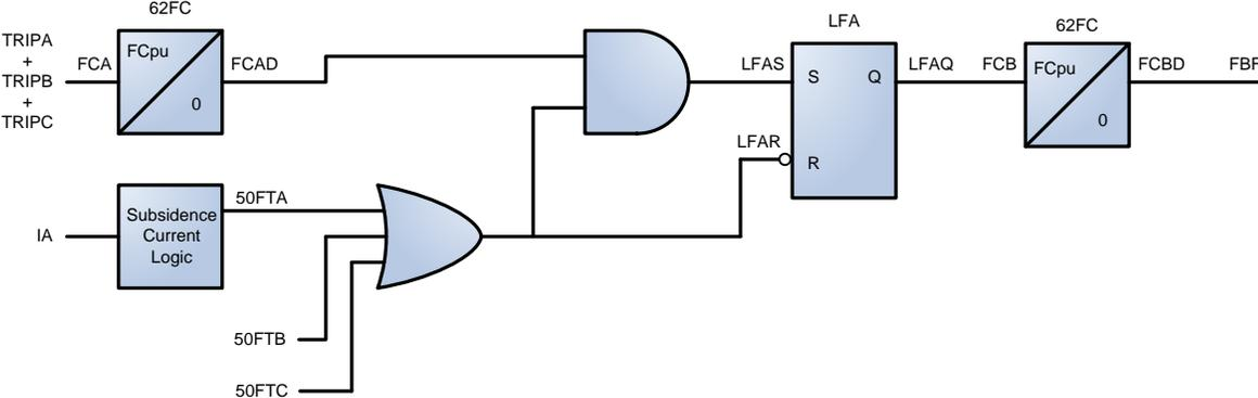
Figure 4: Customized Breaker Failure Scheme
